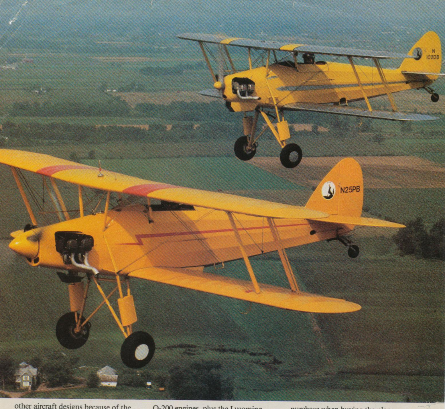
other aircraft designs because of the Skyote's small bays, stepped longerons and boxed-in wing fittings. Basically, the fuselage is a truss structure of welded 4130N chrome-molybdenum steel tubing with wood formers, wood turtleback and fabric covering. Tail surfaces are fabric-covered 4130 steel tubular structures with wire bracing. The stabilizer incorporates groundadjustable incidence but no trim tabs are fitted to the elevators.
