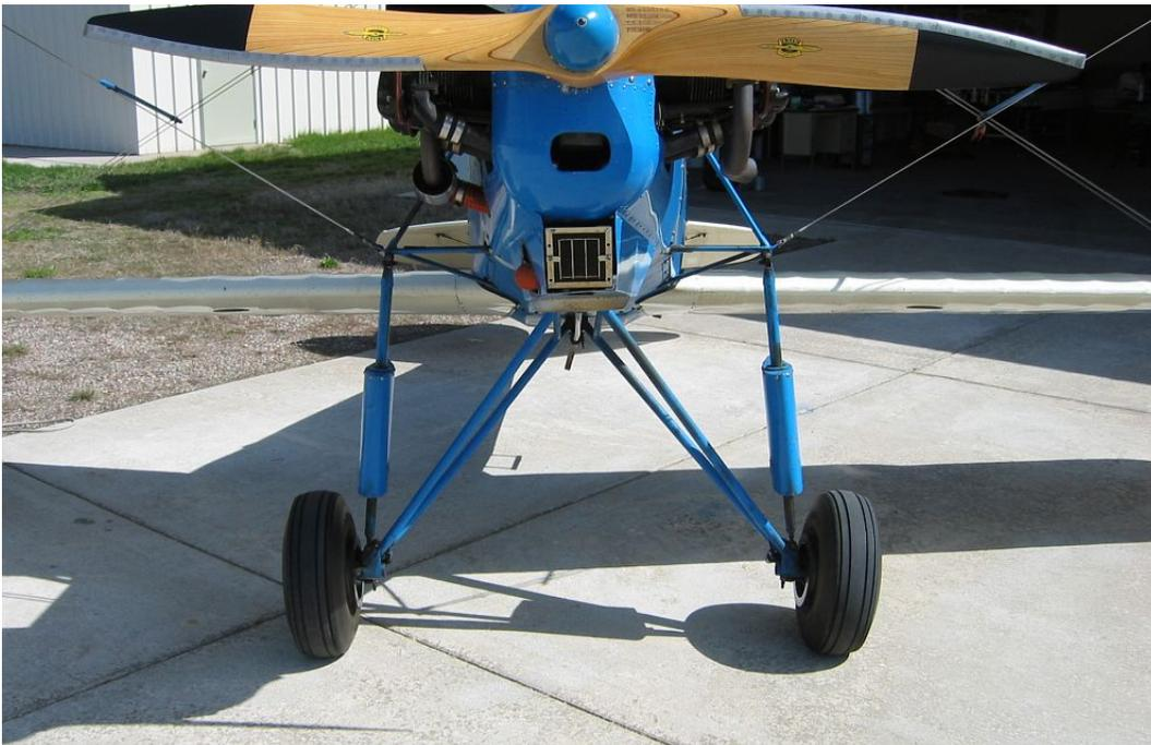
Because the axle is a single piece, there is no easy way to shim-out the alignment errors (see Picture 3 below). Bending the gear would probably have to be done with a lot of heating, and I have not wanted to tackle this because of the inevitable damage to the gear leg fairings. However, when redoing the gear I plan to cut off each axle outboard of
