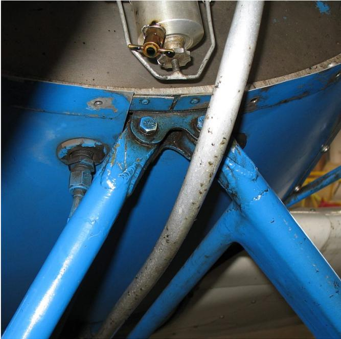
Because of the acute angle geometry of the gear members in this area, these fittings take a real beating during any rough surface operations. Drilling the tabs up one size and fitting stepped replaceable bushings should make repairing the effects of wear a lot easier. There are probably other ways to improve the installation, perhaps edge-welding a large washer onto the face of each of the tabs to increase the bearing areas of the holes.
