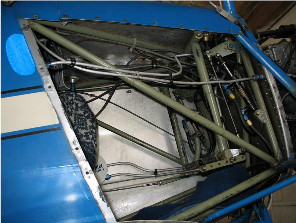
The size of an additional tank suspended below these tubes is limited in the fore-aft dimension by the Rudder Pedal suspension points and cross tube as well as the aft swing of the rudder pedals themselves. The depth is compromised by the reduced head pressure which will result as the bottom of the tank is lowered.
